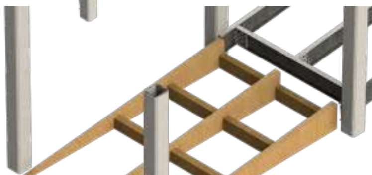
For the deckboards to run to the floor, a bespoke timber structure will need to be fabricated to do so. Ensure there is sufficient room to fix into the posts and suitable joists for the deckboard to fix to
