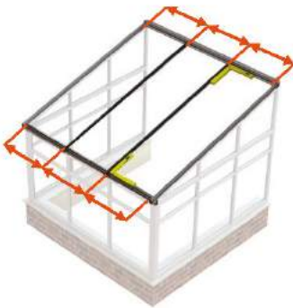
Transom Bar Assembly Section 3.09, pages 24-25
