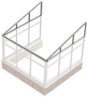
Raked Frame Assembly Section 3.04, pages 14-15
