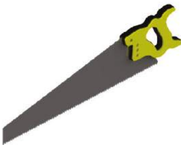
Hand Saw Notching frames
