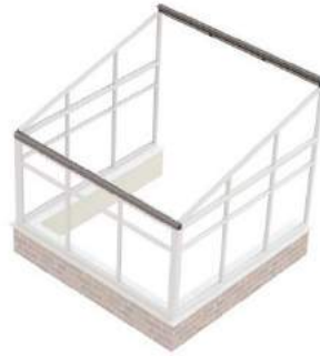
Wallplate / Half Ridge Assembly Section 3.06, pages 18-19 Section 3.07, pages 20-21
