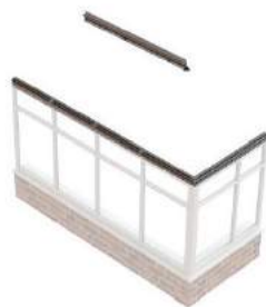
Wallplate / Half Ridge Assembly Section 3.03, pages 12-13
