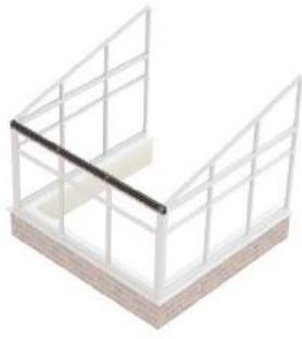
Glazing Retainer Assembly Section 3.05, pages 16-17
