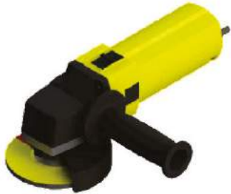
Angle Grinder Chasing out masonry for flashing
