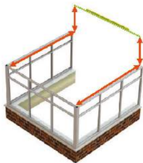
Scribing Half Ridge / Wallplate position Section 3.01, pages 8-9
