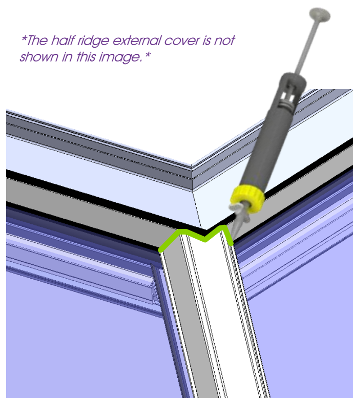
Once fitted in place run a continuous bead of an appropriate sealant along the edge of the hip bar top cap that meets the wallplate / half ridge.
