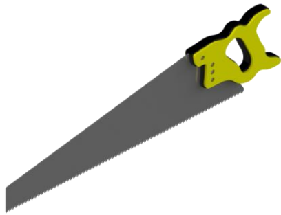
Hand Saw Notching frames
